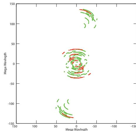
**Fig. 1.** The  $u-v$  plane coverage of EVN network (Megawavelengths) obtained from the observation of source 0234+285, in the e-VLBI experiment EG069C, by red dots are marked the baselines formed by the RT-32 radiotelescope
