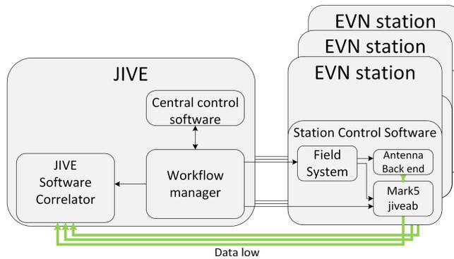
**Fig. 2.** The schema of communication routes and the data flows in e-VLBI session in EVN
