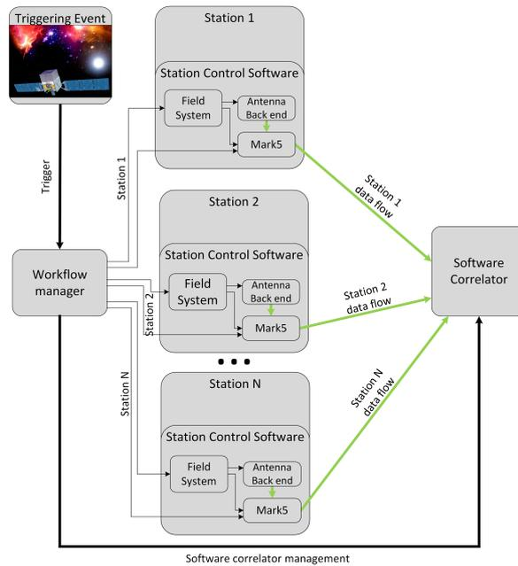
**Fig. 8.** Schematic of triggered e-VLBI observations
