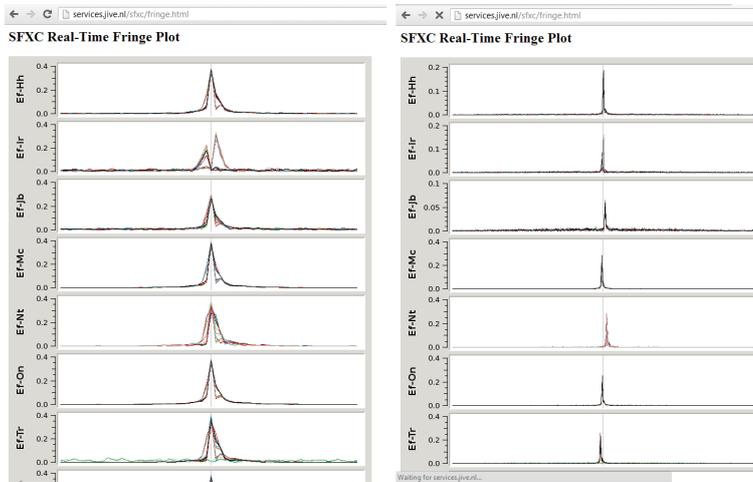
**Fig. 4.** Two snapshots of the real-time fringe plots calculated with SFXC correlator in JIVE during EG069C experiment. The second snapshot (from the top) is displayed the results of the correlation functions of the baseline Effelsberg – Irbene (Ef – Ir). (services.jive.nl/sfxc/fringe.html)
