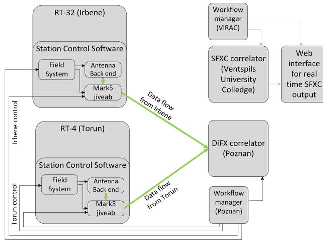
**Fig. 7.** e-VLBI experiment. Data flow from the Torun RT-4 and the Irbene RT-32 correlated in PSNC DiFX correlator. Experiment managed by PSNC operator
