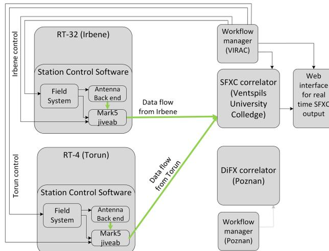
**Fig. 6.** e-VLBI experiment. Data flow from the Torun RT-4 and the Irbene RT-32 correlated in VIRAC SFXC correlator. Experiment managed by VIRAC operator
