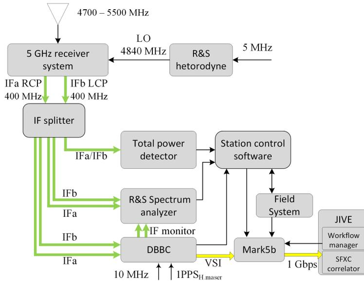
**Fig. 3.** Connection scheme of receiving and recording equipment for e-VLBI experiments at the RT - 32
